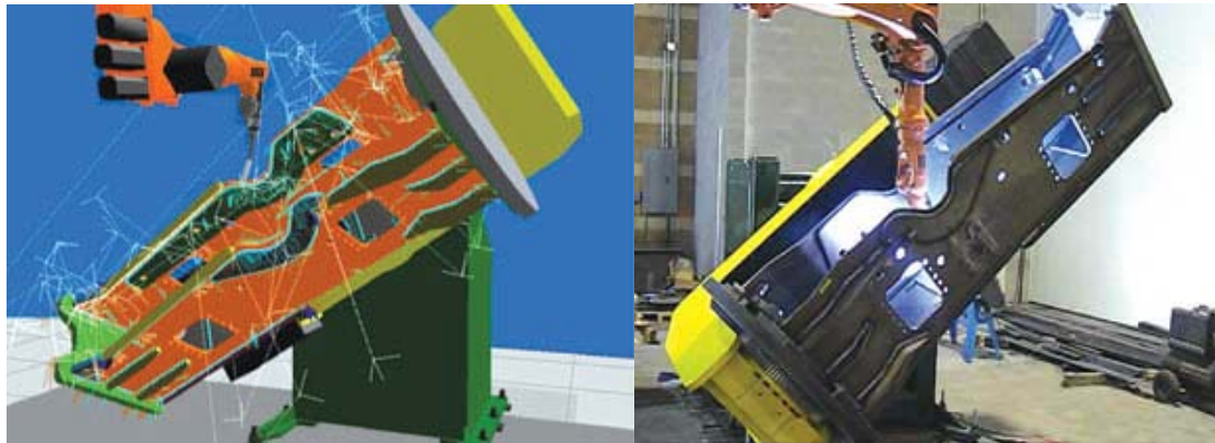
A new robot developed for low-volume applications programs itself within hours using a CAD drawing, then welds the final part.
